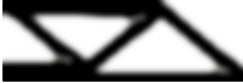
Figure 7: Optimal design for the MBB problem
