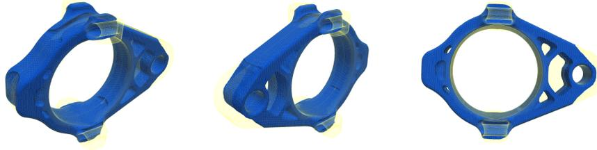
Figure 11: Topology optimization results of the clasp in PLA.
